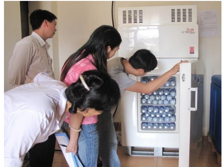
Solar powered refrigerator in Vietnam.
