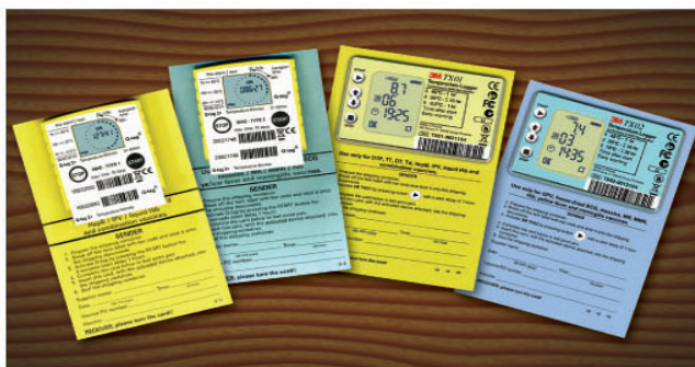
10-day electronic temperature monitoring devices show when, and to what extent, the set temperature conditions have been violated.
