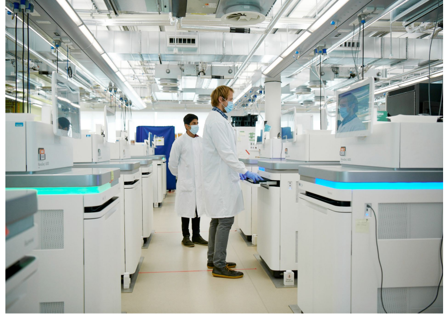
7 Illumina Novaseq - 10k samples per machine. Average 2.5M reads per sample
