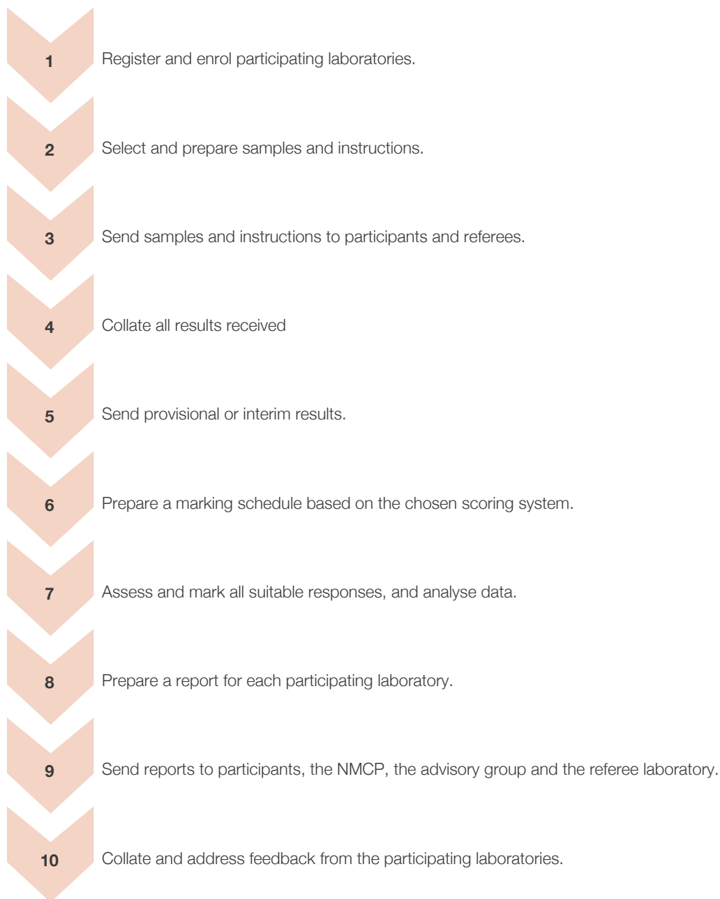
Figure 7. Flow of activities of the proficiency testing provider
