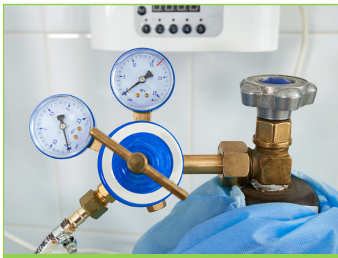
Imagen 5: Oxygen regulator for gas cylinder. The cylinder valve regulates the gas coming out of the cylinder (pressure gauge closest to the cylinder) and the regulator controls the gas entering the circuit (pressure gauge on the left). This picture shows how the polyamide tube is connected directly to the regulator.
