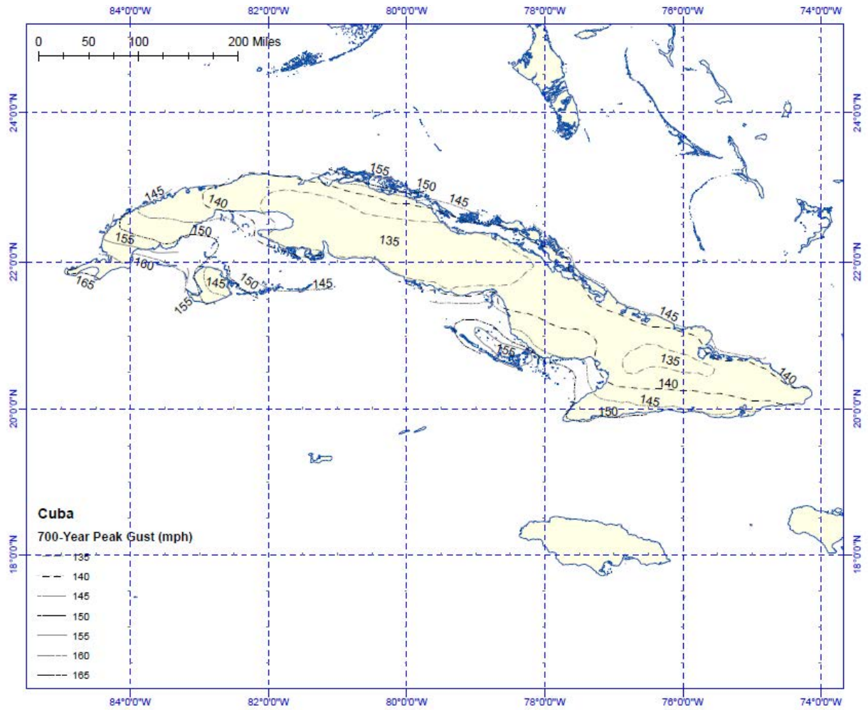
Figure 3-14. Contours of predicted 700-year return period wind speeds (mph) at a height of 10 m above flat open terrain for Cuba.
